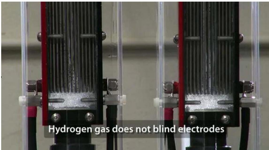
*The clear design of the electrolytic cells allows the operator to see what is happening. The degree of scaling, an indication of need for cell cleaning, can also be easily observed.*
