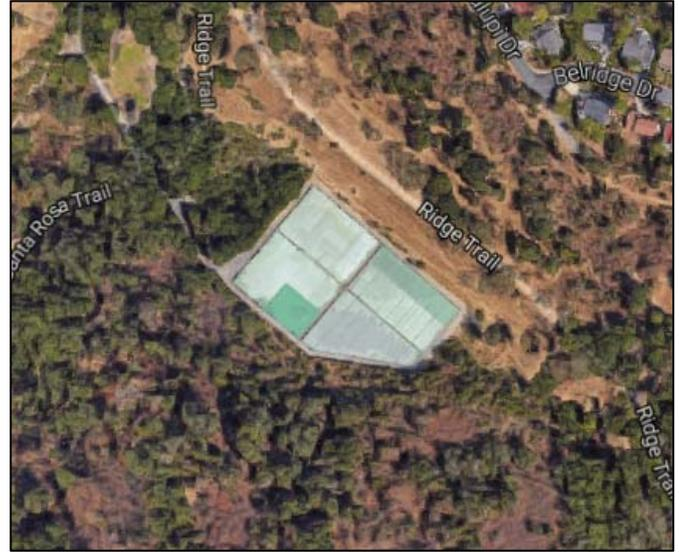
The design of the new reservoirs posed a unique challenge as the Department of Drinking Water (DDW) in California requires dedicated inlet and outlet lines for any new reservoir in an effort to maintain water quality by avoiding “short-circuiting” within a tank. However, the seismic considerations combined with the proposed location of the new Belgatos Reservoirs would have made the addition of dedicated inlet/outlet lines for each tank costly from an engineering and construction perspective.
